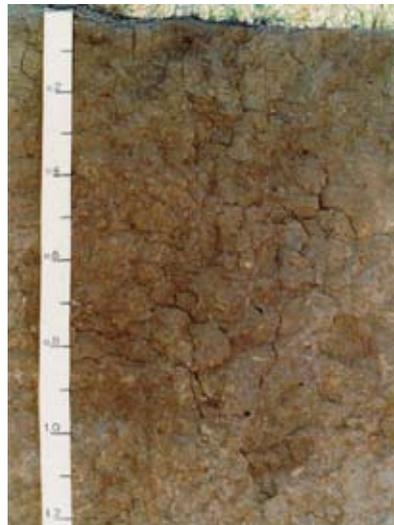
An example of a clay profile. Slowly permeable, imperfectly drained, retains high amounts of water.
