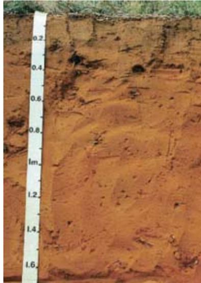
An example of a sand profile. Highly permeable, excessively drained, retains only low amounts of water.
